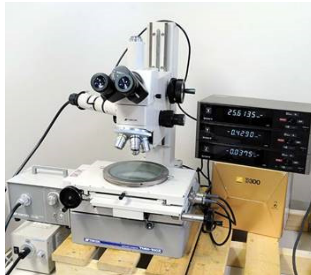
Microscope: Topcon TMM-130Z Measuring range: 130 x 130 x 50 mm Minimum indication: 0.001 mm Accuracy: (3 + 2.5L/100) \mu\text{m}
