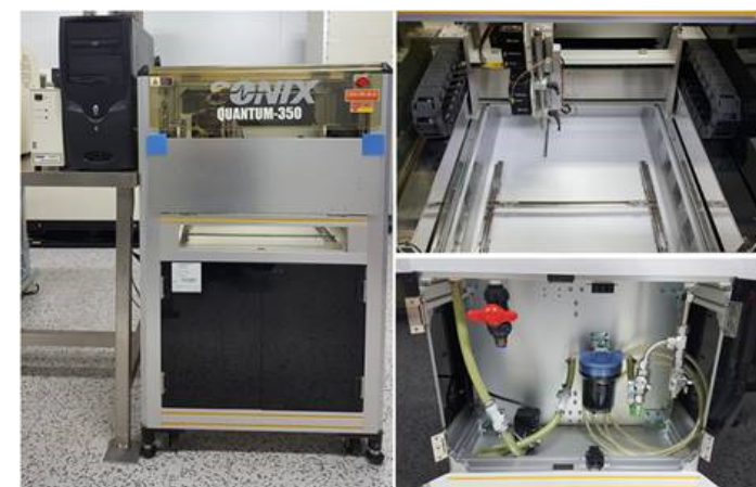
C-SAM: Sonix Quantum 350H Spatial resolution:0.5 µm Depth resolution: 8 µm
